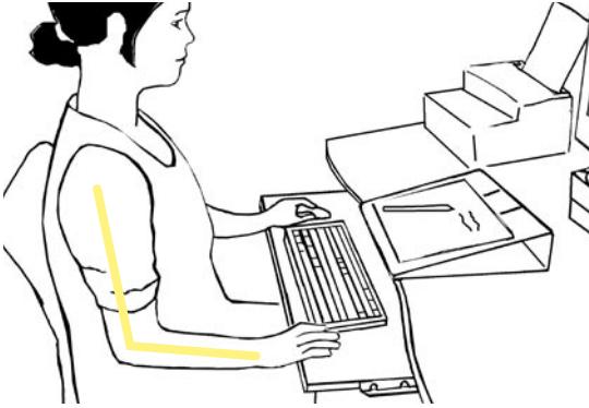
The keyboard is correctly placed: about 5 cm lower than the elbow when the arm is suspended from the shoulder
